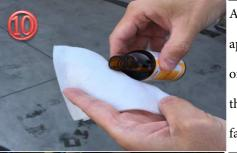
Apply the appropriate amount of headlight coat II to the non-woven fabric.
